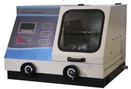
XCut-349/350 cutting machine is composed of main unit, electric control box, cutting room, motor, cooling system, cutting wheel and other parts.
